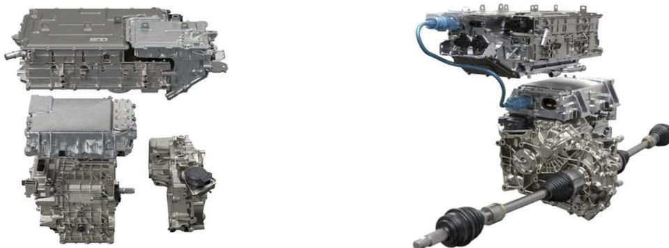
Thanks to its optimised design, the engine is compact and only weighs 145 kg (clutch included), that is 10% less than the engine currently used on ZOE, despite a marked increase in both power and torque. Each All-new Mégane E-TECH Electric will be fitted with one of following:
