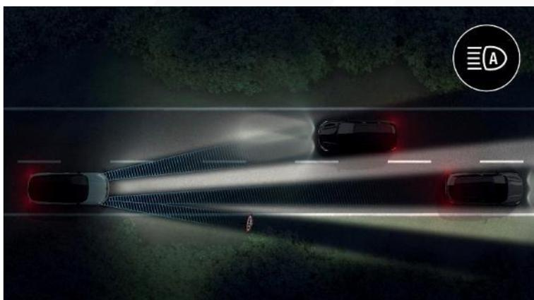
The **Matrix LED Vision** (Matrix beam / ADB) means drivers can continue using high beam for the greatest coverage no matter what the surrounding traffic is like. This is made possible thanks to anti-glare LED technology that adapts the direction of light beams to ensure the comfort and safety all those in nearby vehicles.
