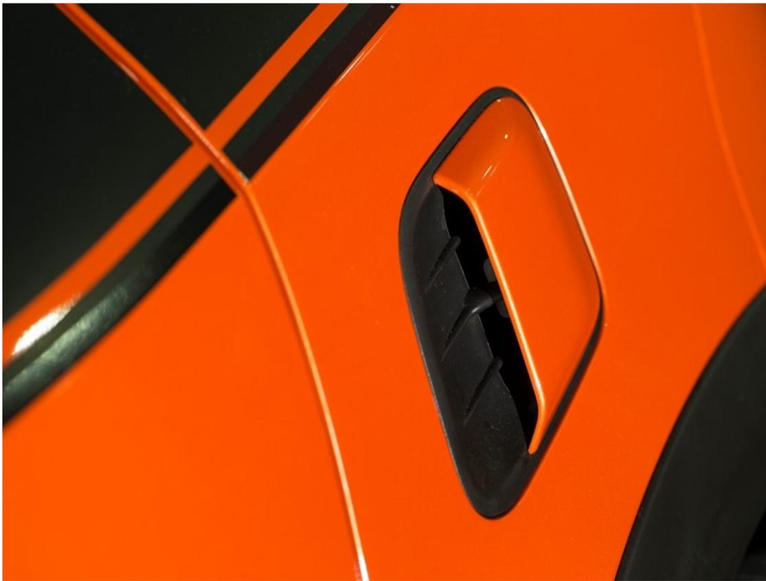
One of TWINGO GT's distinctive features is the air intake on the rear left-hand wing, which replaces the air intake that was originally located above the wheel arch. This modification is essential in improving engine performance, since it reduces the temperature of the air entering the turbocharger by some 12%. Combined with an upper section duct, this dynamic intake also helps increase the flow rate of combustive air by 23%.
