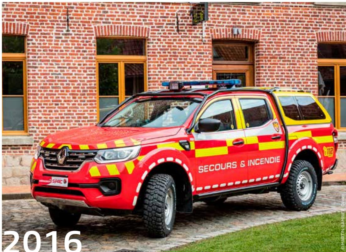
This is a strong, powerful one-tone pick-up with exceptional off-road ability. It is both robust and exceptionally comfortable, with its five-link rear suspension and strong ladder-frame chassis.
