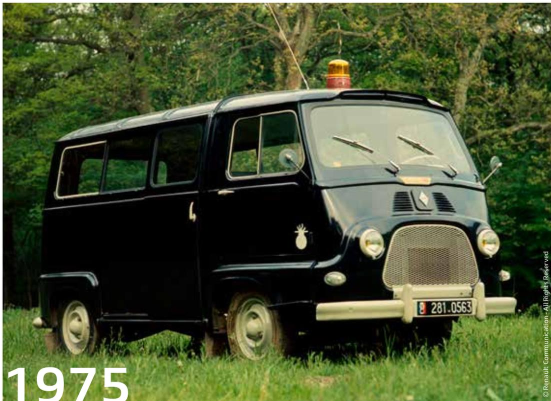
Renault's first front-wheel drive car was a small commercial vehicle. The Estafette has a flat floor, independent wheels, a very short turning circle and sliding doors on the driver side.
