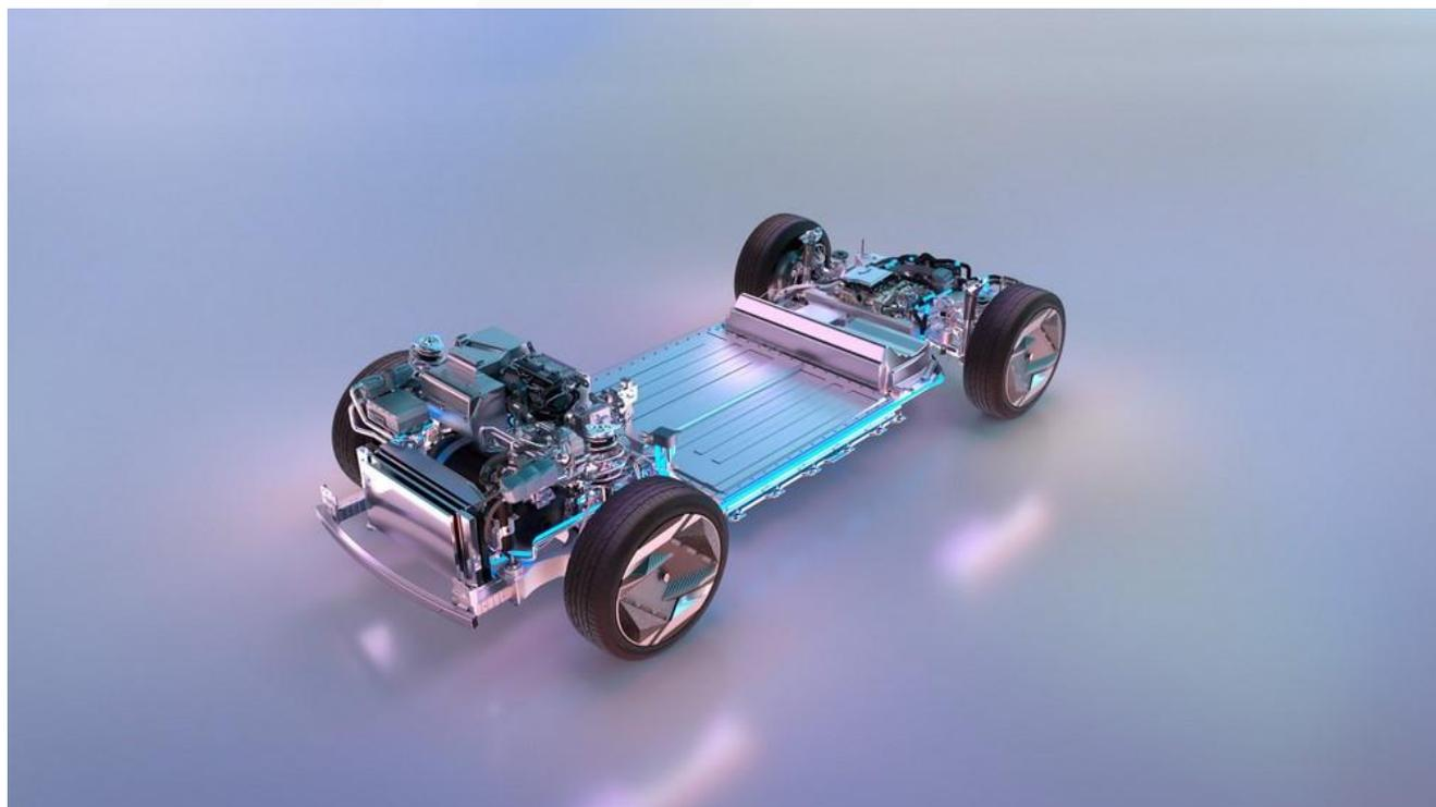
Renault Scenic Vision's 160 kW electrically excited synchronous motor derives directly from All-new Renault Megane E-TECH Electric's motor and is made at the plant in Cl on. It uses no rare-earth elements, which helps to reduce its carbon footprint and create a responsible and sustainable ecosystem. The 40 kWh battery is recyclable and will be made in France by 2024 at the Renault ElectriCity Gigafactory. It is
