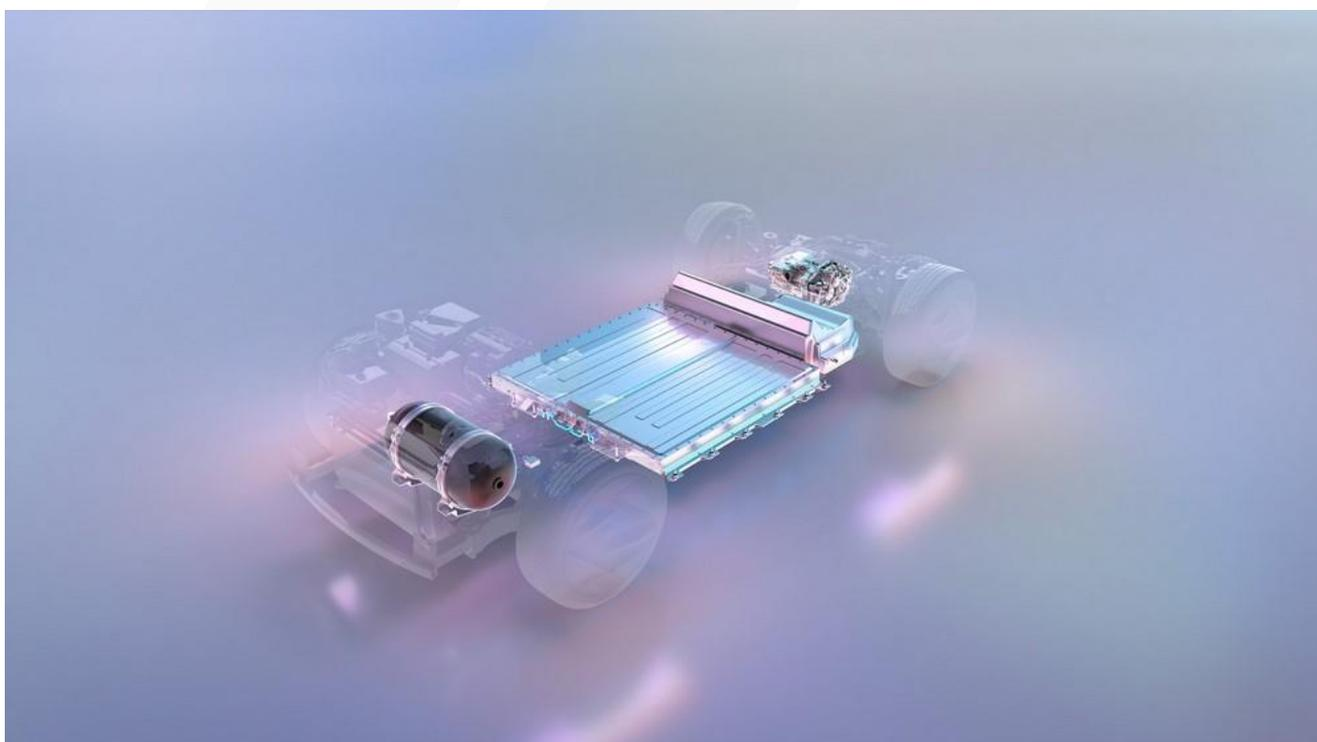
Renault Scenic Vision has an all-new platform that is purpose-designed to fit all the components: the electric motor, hydrogen engine, battery, fuel cell and hydrogen tank. The engine is at the rear, so there is enough space for the 2.5 kg hydrogen tank at the front; the fuel cell is under the floor, at the back of the platform, behind the battery.
