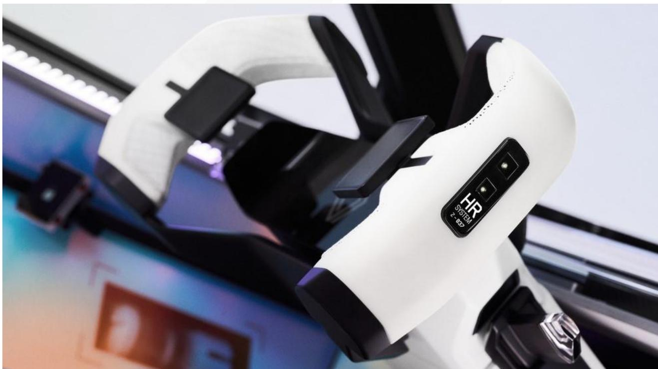
To further drivers, the vehicle comes fitted with an array of health monitoring systems. A heart rate sensor placed in the steering wheel and a camera serve to detect signs of driver fatigue or idleness. Should a problem arise, warning signals are sent to the driver and passengers.
