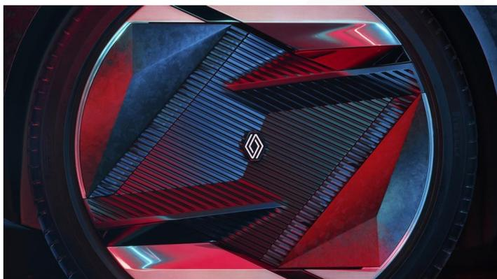
Fitted with large 21-inch wheels, the rims on the Renault Scenic Vision are equipped with flaps for enhanced aerodynamic performance, and therefore greater efficiency. When the car is in motion ( $\geq 10\text{km/h}$ ), the flaps close to improve their aerodynamics; as soon as the car slows down and its speed drops below  $10\text{km/h}$ , the flaps open for better cooling as the heat generated by the brakes can escape more readily.
