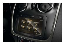
Making its debut on Dacia Lodgy and Dokker, MEDIA NAV is available on all three new models. The simple and user-friendly system, fitted seamlessly in the central fascia, comprises in-car navigation, a radio, Bluetooth® handsfree kit connection and audio streaming, all controlled via a 7-inch (18-cm) touch screen. Navigating the system is
